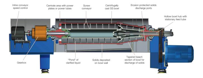
SG2 decanter design and working principle
